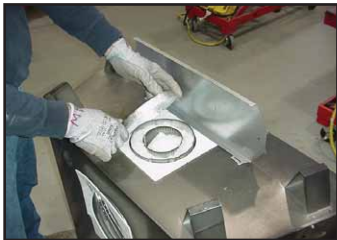
Figure 9.4 Remove the seal cap.
